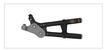
The Torq Tool is lightweight, compact, and works with all sizes of Gripple Plus joiners to tension the fence wire. Designed with a built-in-gauge, the tool measures the tension you wish to apply.
