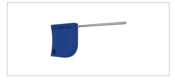
The Setting Key allows Gripple tensioners to be repositioned on the wire before tension is applied. To use, simply insert the key into the small hole adjacent to the main channel, releasing the roller and allowing the Gripple to move freely.
