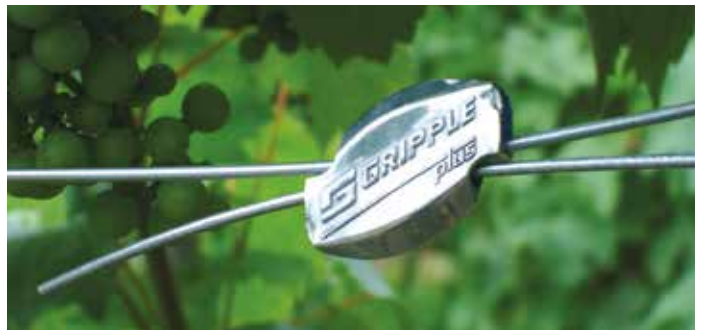
Top: Wire repair using GP Medium tensioning with Torq Tool; Bottom: Standard join of trellis wire
